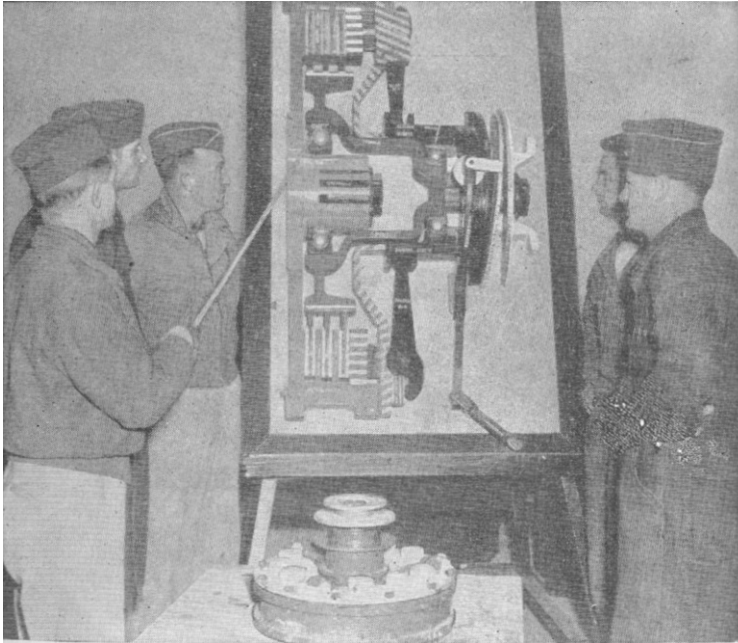
FIGURE 21.—Sectionalized enlarged model of clutch mechanism used in conjunction with object.
