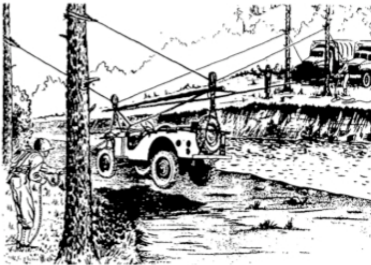
Figure 15. Aerial cableway showing movement of \frac{3}{4} -ton truck by double-cable crossing.
