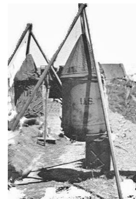
“Lister bag”, invented by Army Surgeon William Lyster. Water is loaded from the top and treated with Calcium Hypochlorite to render it potable. Introduced in 1917.
