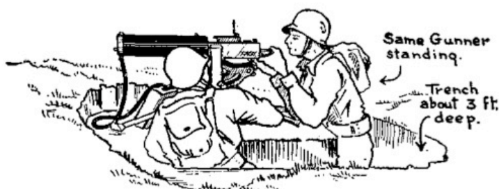
FIGURE 31.—Standing type heavy machine-gun emplacement.
