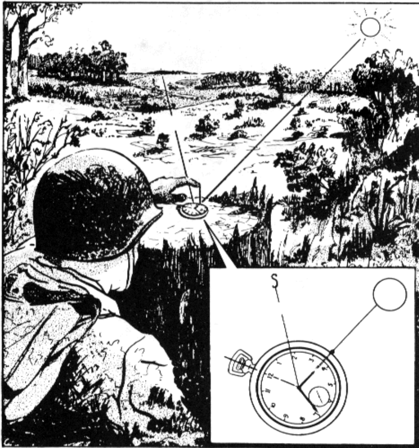
Figure 9. Sun and watch method of determining direction.
