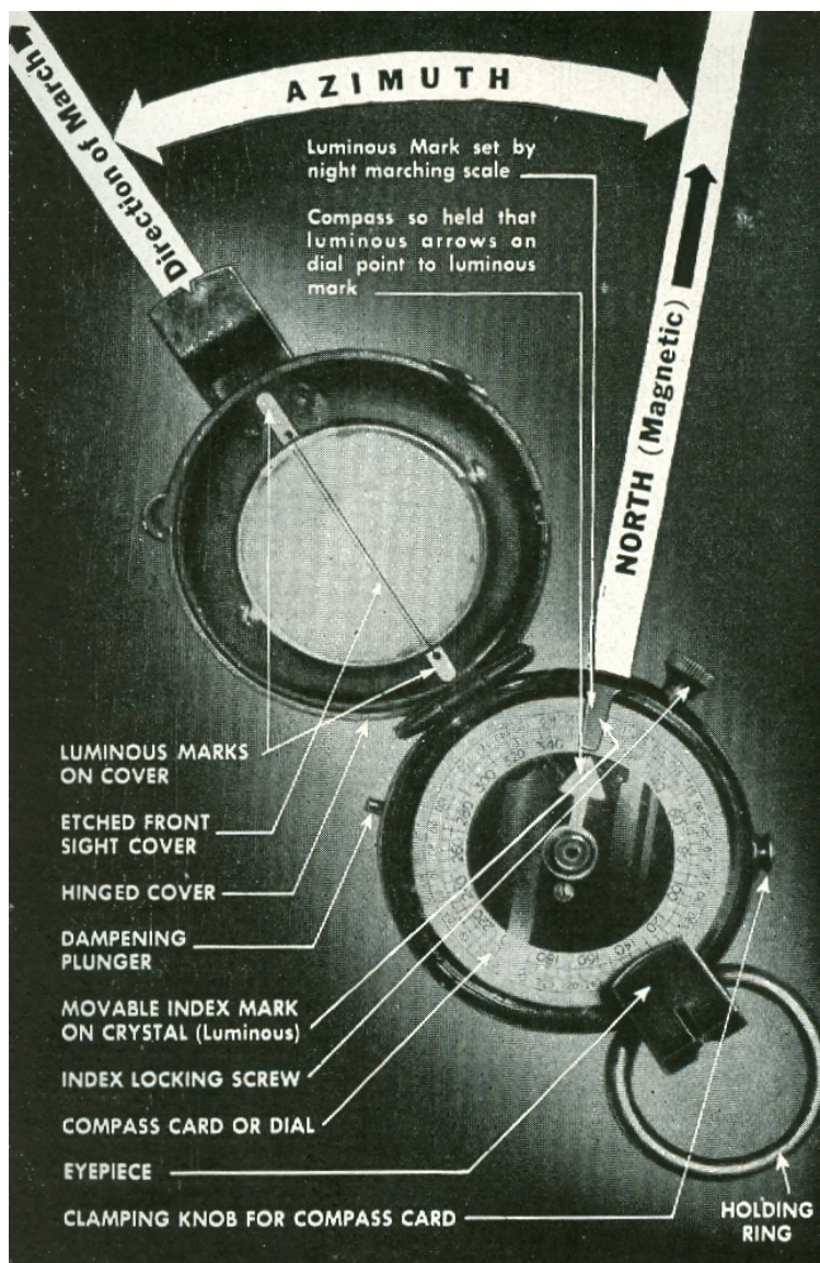
Figure 19. Nomenclature of prismatic compass.
