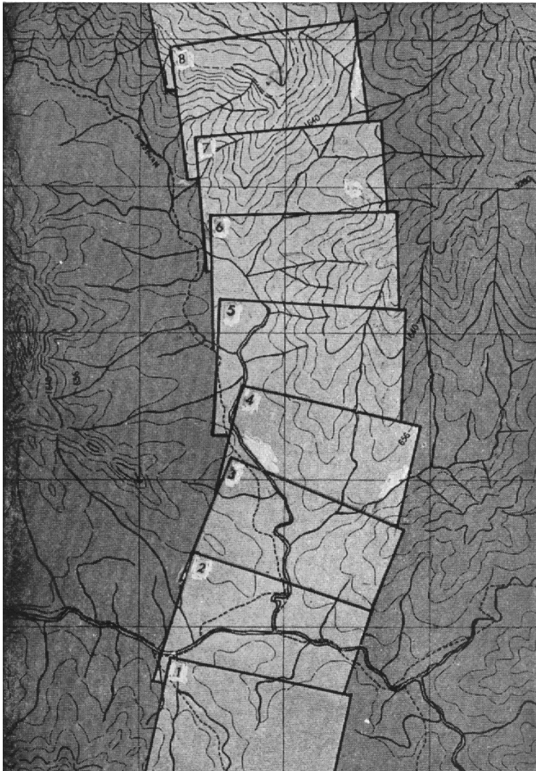
Fig 67. Line diagram showing relative positions of separate pictures in a photographic strip.
