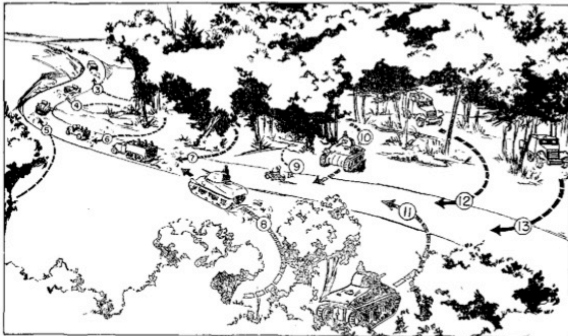
FIGURE 15.—Move vehicles out and form column moving.
