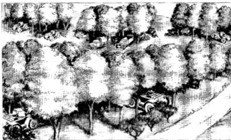
② Select an area big enough to permit maintenance, supply, and command vehicles to fit in without crowding.
